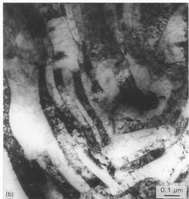
Figure 4(a, b) TEM bright-field micrographs of Path I Ti-50Y extruded at 860 °C to  $\eta = 2.8$  and hot swaged at 725 °C to  $\eta = 4.7$ . Mean-free distance between phases in this specimen is 150 nm.
