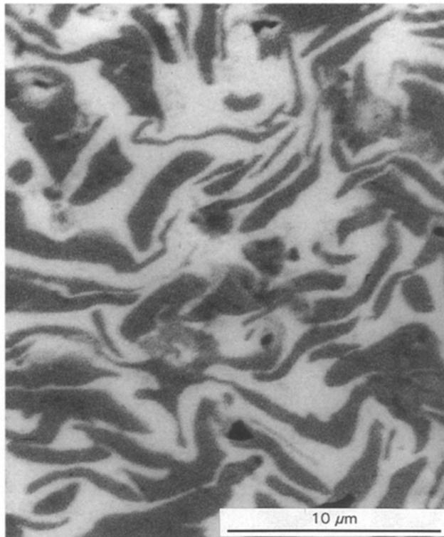
Figure 2 SEM back-scattered electron micrograph of a transverse section of Ti-50Y extruded at 860 °C to  $\eta = 2.8$ . Mean-free distance between phases in this specimen is 890 nm.
